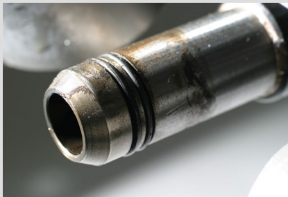
The O-rings on the filter pan pickup tube should be changed regularly.
