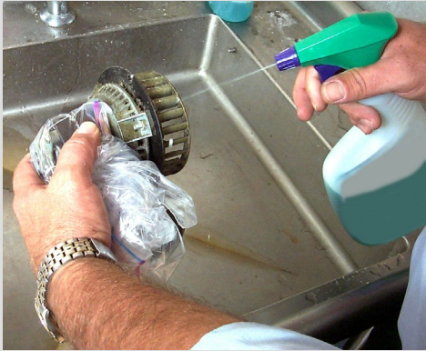
Cleaning the blower motor ensures even combustion.
